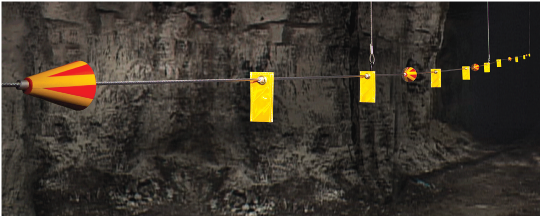
CAB Extra High Visibility Lifeline is easily seen from any direction in escapeways. Lifeline markers hang vertically so they can be seen for long distances up and down escapeways. Markers are flexible so miners' hands can slide easily over them.
