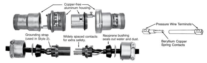
**Energized contacts** deeply recessed to reduce danger of accidental touching, minimize possibility of exposed arcs. Insulator quenches arcing, and is resistant to abnormal heat and to fire.
