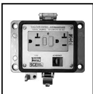
RJ-45 CAT5 F/F connector with 120 VAC Duplex GFCI with internal Simplex GFCI. No circuit breaker
