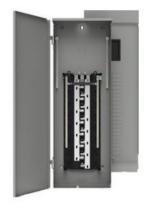
SIEMENS LOW VOLTAGE PL SERIES LOAD CENTER. MAIN LUG WITH 42 1-INCH SPACES ALLOWING MAX 60 CIRCUITS. 3-PHASE 4-WIRE SYSTEM RATED 120/240V OR 120/208V (225A) 100KA INTERRUPT. SPECIAL FEATURES: COPPER BUS, INTERCHANGEABLE MAIN, GRAY TRIM, NEMA TYPE3R ENCLOSURE FOR OUTDOOR USE.
