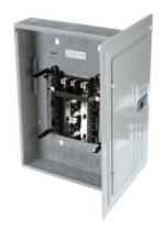
SIEMENS LOW VOLTAGE PL SERIES LOAD CENTER. MAIN LUG WITH 12 1-INCH SPACES ALLOWING MAX 24 CIRCUITS. 3-PHASE 4-WIRE SYSTEM RATED 120/240V OR 120/208V (125A) 100KA INTERRUPT. SPECIAL FEATURES: COPPER BUS, INTERCHANGEABLE MAIN, GRAY TRIM, NEMA TYPE1 ENCLOSURE FOR INDOOR USE.
