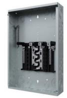
SIEMENS LOW VOLTAGE PLUG-ON NEUTRAL READY STANDARD SERIES ASSEMBLED LOAD CENTER. MAIN LUG WITH 12 1-INCH SPACES ALLOWING MAX 24 CIRCUITS. 1-PHASE 3-WIRE SYSTEM RATED 120/240V (200A) 100KAIC. SPECIAL FEATURES: ALUMINUM BUS, GREY TRIM NEMA TYPE 1 ENCLOSURE FOR INDOOR USE.
